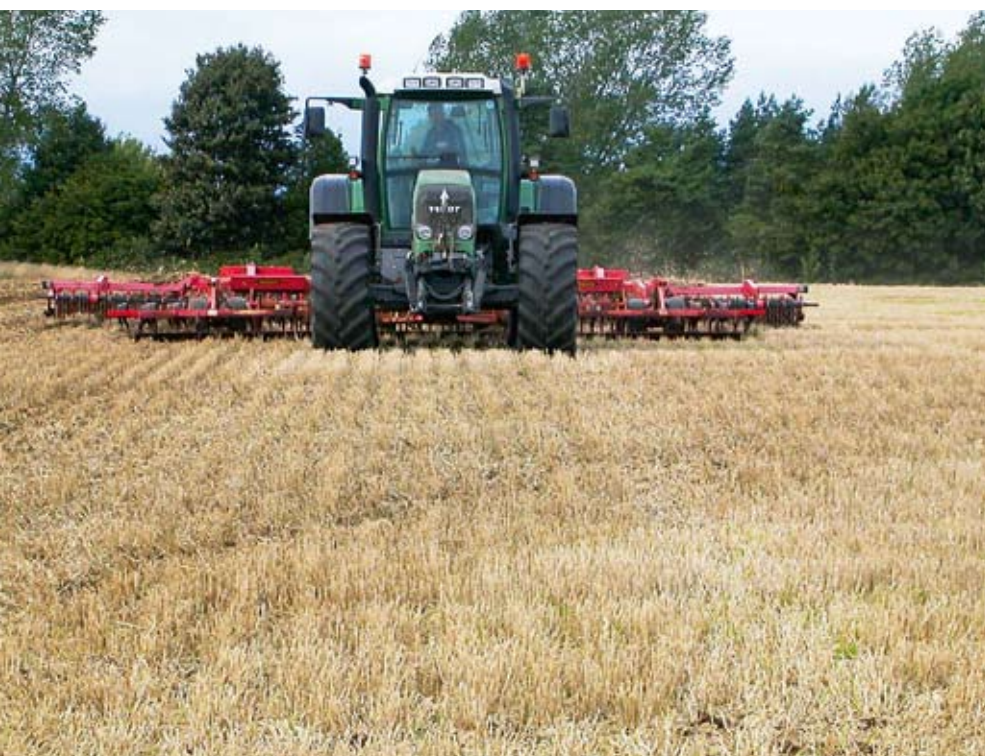
The farm's Fendt 820 tractor was ordered with a 2m track width to fit the Out Track controlled-traffic farming system. Here the tractor's wheels are in the combine's marks, in between the farm's 22m tramlines.
