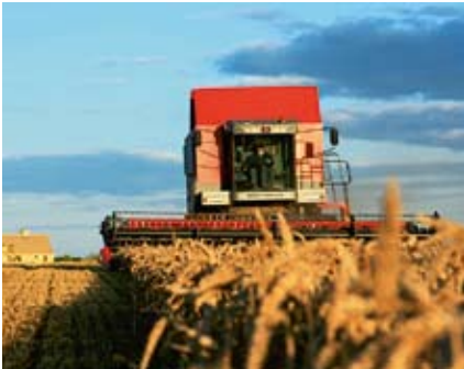
Nick August based his Out Track controlled-traffic system around his MF 7274 Cerea's 7.5m header. He couldn't justify changing his combine just to fit in with CTF.
