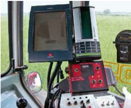
The LH 5000 controller is used on the sprayer and spreader. Massey's Datavision II+ screen plays a part in both mapping and controlling variable rates.
