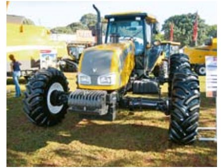
This 'special' Valtra is designed for a system in which all the tractors and vehicles run in the same tracks. Out Track avoids this specialist machine mod cost.
