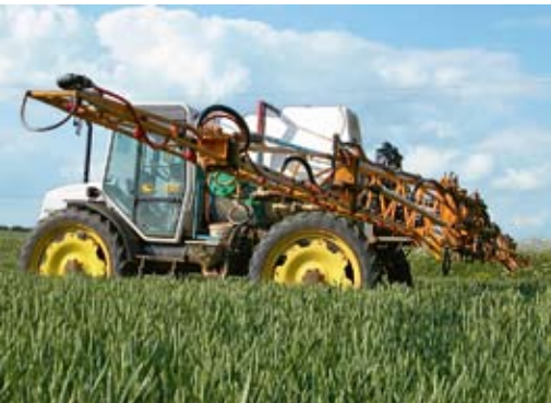
The original 20m booms on the Clayton C410S were extended with the addition of 1m long sections at each end. The machine now fits into the 22m wide system.
